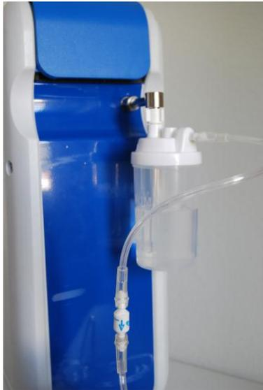
Fig. 39: Connection with the humidifier
