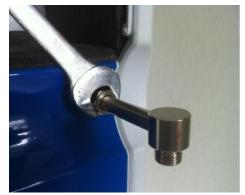
Fig. 34: Angle connection
