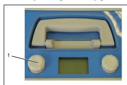
Fig. 52: Adjusting the volume flow
