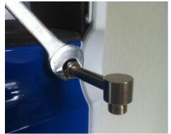
**2 Screw the angle connection** to the oxygen outlet of the Kröber O2 4.0 with a wrench (metric size 17).
